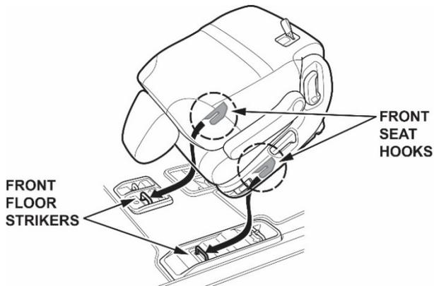
2. Slide the seat into either the standard or wide position:
